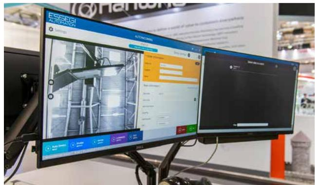
An image of each component and barcodes is stored in the database and is available for future recall for visualization and quality checking. This tool brings traceability to an even higher level and it can also provide evidence of damaged or mislabeled material coming from suppliers.
