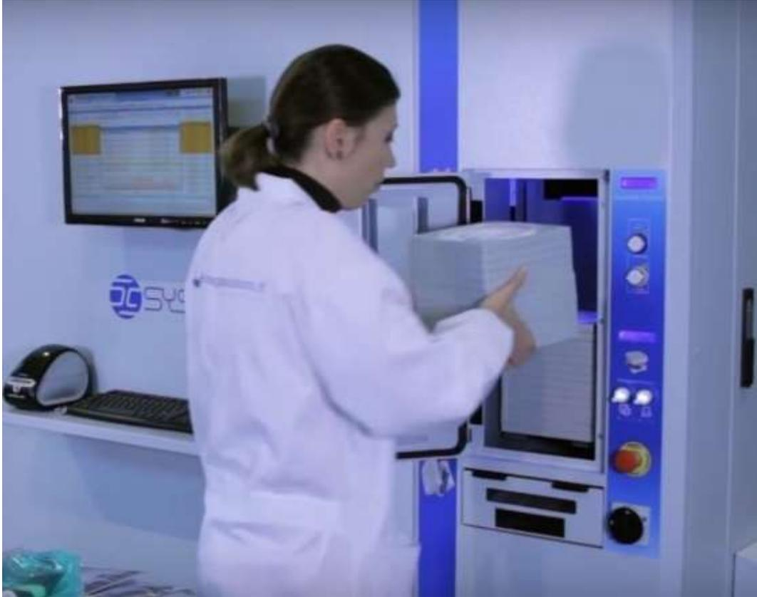
**An operator removes a stacked kit from an Essegi Tower**
